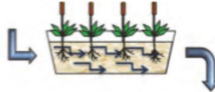
Horizontal subsurface flow (HSSF)
